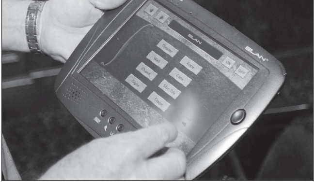
Gary Sorley works the system that controls the curtains, sound, lights and the movie on the screen.
